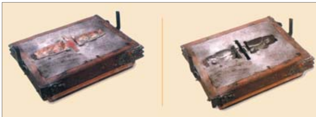
1. Shaping the Sand : A wooden pattern cut to the shape of one half of the casting is positioned in an iron box and surrounded by tightly packed moist sand.
